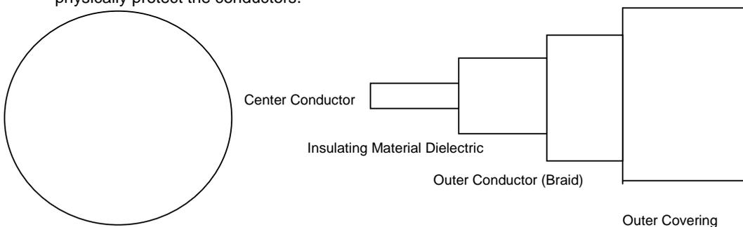
The center conductor is the primary means of carrying a video signal. The center conductor generally solid copper is available in varying diameter. Cable with large diameter center conductor have lower resistance than cable with smaller diameters and enhances the ability of a cable to carry a video signal over a longer distance with better clarity.
